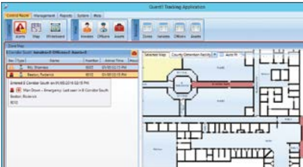
Zone-based tracking displays the alert location
